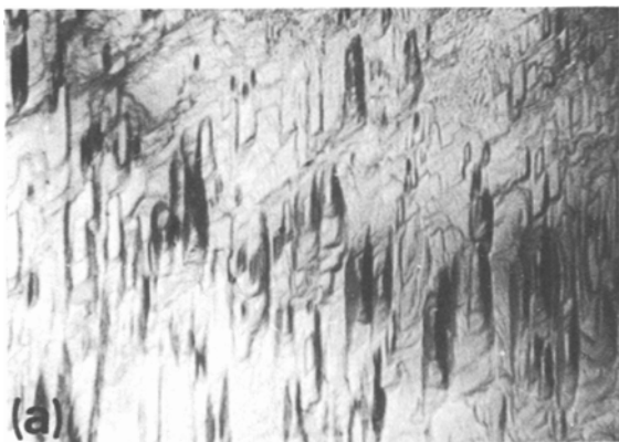
Figure 2 Etch pits produced on the (010) surface of KDP by (a) H_2O , (b) CH_3OH and (c) CH_3COOH after etching for 2 sec, 4 h and 6 min, respectively. Shallow pits may be seen in (b). The marker indicates 0.3 mm.
